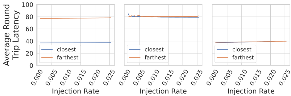
Fig. 12: Impact on Secure LD round trip latency on (a) Baseline (b) CAMOUFLAGE JITTER (c) CAMOUFLAGE BYPASS policies
