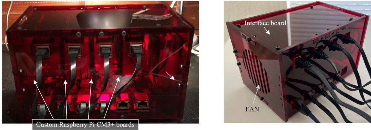
Figure 4. Enclosure and assembled RPi compute module 3 cluster.
